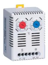
Two thermostats in one casing. Thermostat (contact breaker, normally closed) for regulating heaters. The contact opens when temperature is rising. Thermostat (contact maker, normally open) for regulating filter fans and heat exchangers or switching signal devices when temperature limit has been exceeded. The contact closes when temperature is rising. heaters and cooling equipment can be switched independently from each other with a temperature offset as opposed to the usual change-over contacts.
