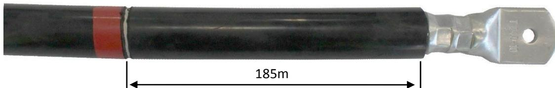
Using a file, ensure black semi-conductive sheath is rounded and without sharp edges.
