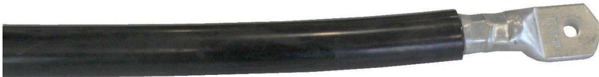
3. Using tape, mark the cable 245mm from where black insulation and lug meet. Use a file to strip black outer sheath where marked by tape.
