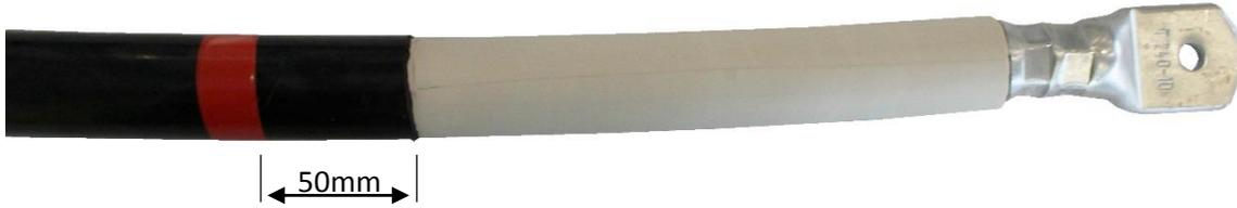
6. Clean the white insulation using the alcohol-based electrical cleaning wipes provided in the termination kit. Once dry, apply silicone lubricant to top of insulation.
