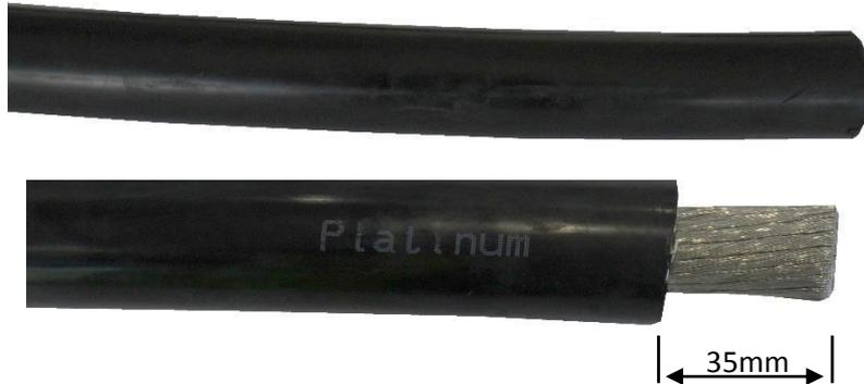
2. Using tape, mark cable 185mm from where black insulation has been stripped. Use a file to strip black outer sheath where marked by tape.
